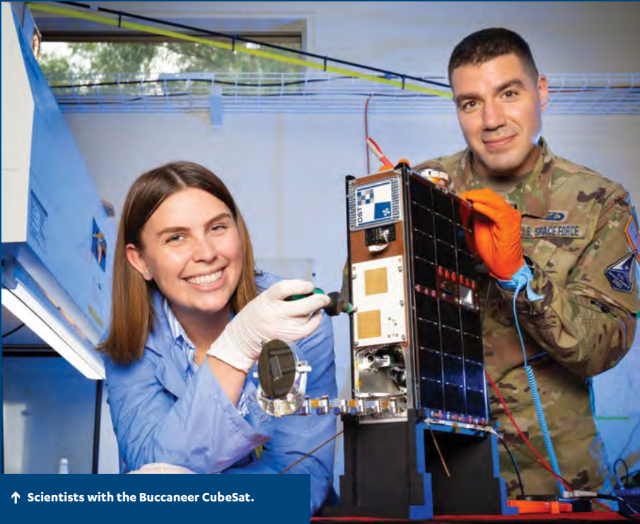
↑ Testing the high-frequency payload on the Buccaneer Main Mission cube-satellite at DSTG Edinburgh.
