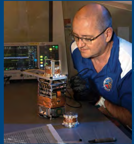
↑ Testing the high-frequency payload on the Buccaneer Main Mission cube-satellite at DSTG Edinburgh.
