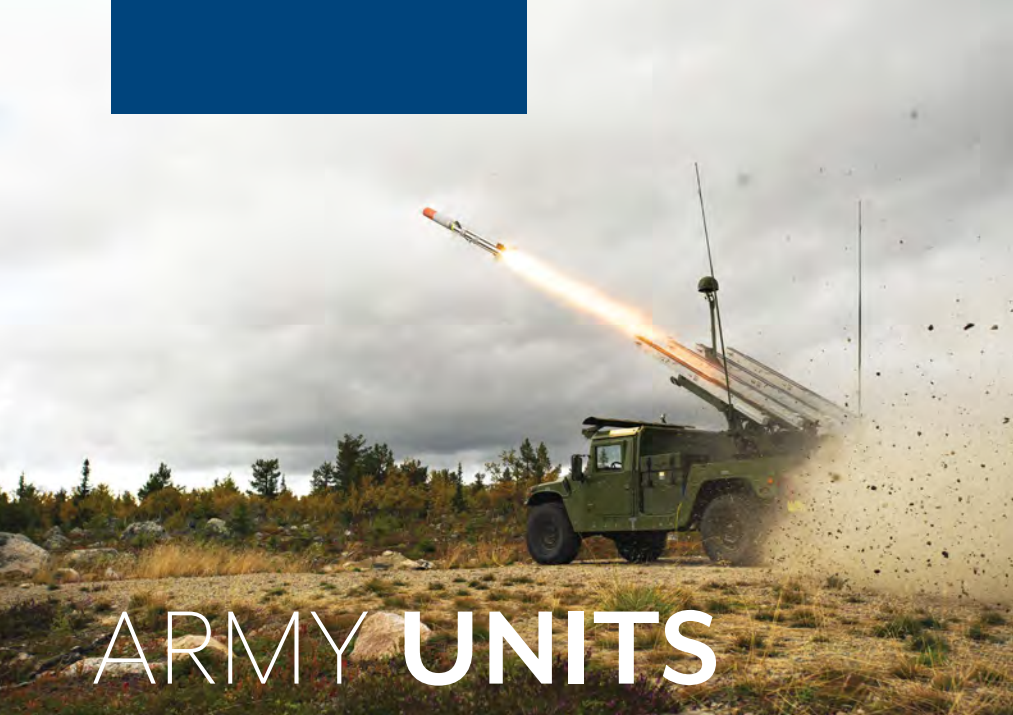
← The NASAMS High Mobility Launcher on a High Mobility Multipurpose Wheeled Vehicle firing an AMRAAM missile.
